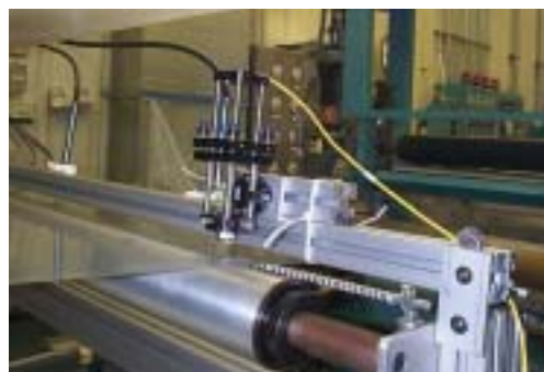
Lumetrics' DI 330 OPTIGAUGE Film Thickness Measurement System employs advanced optical technology to measure coating and complete successful on-line testing with a medical films' manufacturer.
